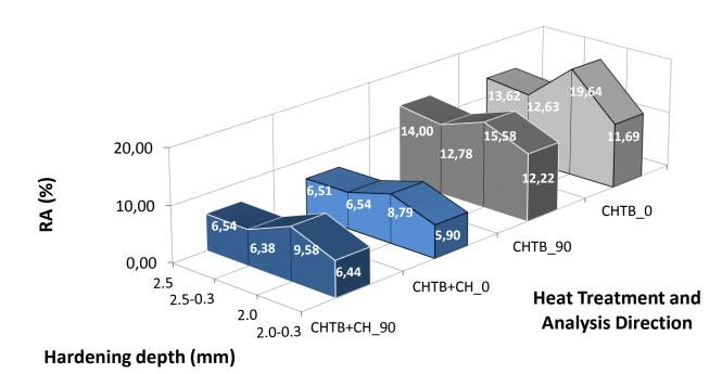
Fig. 2 Retained austenite measurements on of heat-treated UNI 18NiCrMo5 specimens produced by a manufacturing process involving Carburizing, Hardening, Tempering and Blasting (CHTB) and Cryogenic-Hardening (CH) additional step.
