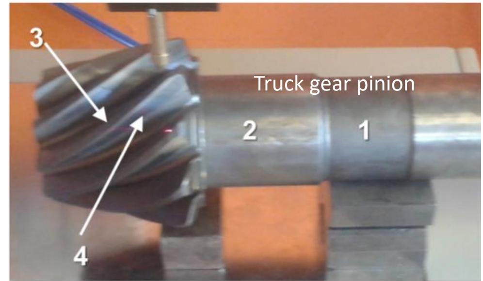
Measurement performed on pitch diameter of a gear.
