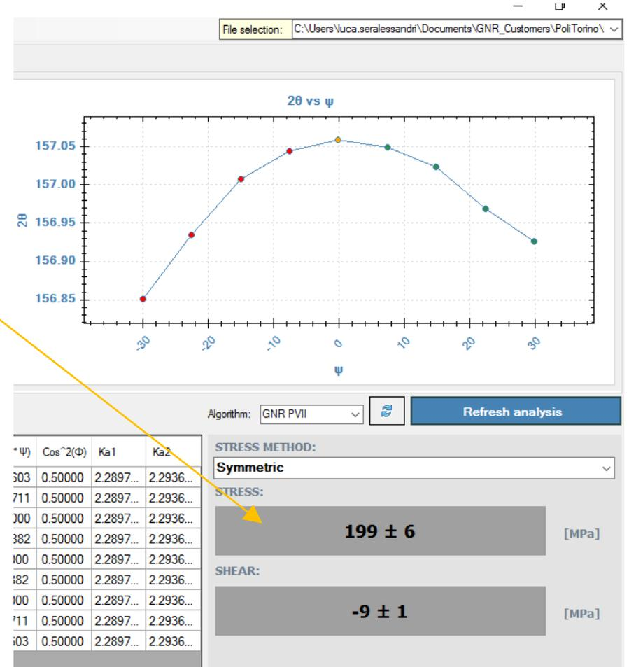
Suspensions: tri-axial analysis of welding, residual stress tensor as input for finite element simulations.
